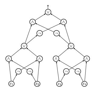
If S(n) is the size of the above circuit for computing parity over n input variables, then S(n) = 2S(n/2) + 5, and S(1) = 1. Solving this recursion, we get S(n) = O(n), as desired.
