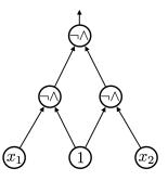
Any circuit with AND, OR, and NOT gates can be converted to a one using only NAND gates by replacing each AND, OR, and NOT gate with the corresponding circuit as shown above. For each gate we replace, we need to use at most 3 NAND gates. So the size of our circuit with NAND gates will be at most 3 times as the size of the original circuit.
