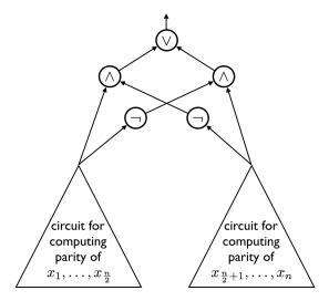
Note that the gadget above the two triangles is just a circuit computing the parity of two bits. For n = 4, the construction would materialize as follows:
